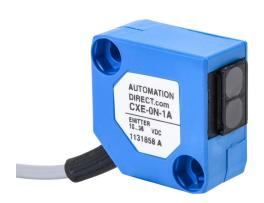
AutomationDirect photoelectric sensor, rectangular, plastic housing, through-beam emitter, infrared light emission, 6m sensing distance, 10-36 VDC operating voltage, 3-wire, pigtail.
