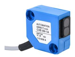
AutomationDirect photoelectric sensor, rectangular, plastic housing, through-beam emitter, infrared, 6m sensing distance, 10-36 VDC operating voltage, 3-wire, pigtail.
