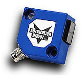
AutomationDirect photoelectric sensor, rectangular, plastic, diffuse with background suppression, 15-150mm sensing distance, light-on, PNP, potentiometer, 500 Hz switching frequency, 3-pin M8 quick-disconnect.
