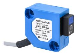
AutomationDirect photoelectric sensor, rectangular, plastic, diffuse with background suppression, 15-150mm sensing distance, light-on, PNP, potentiometer, 500 Hz switching frequency, 6.5ft/2m cable length, pigtail.
