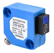
AutomationDirect photoelectric sensor, rectangular, plastic, diffuse with background suppression, 15-150mm sensing distance, light-on, NPN, potentiometer, 500 Hz switching frequency, 3-pin M8 quick-disconnect.
