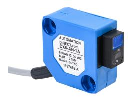
AutomationDirect photoelectric sensor, rectangular, plastic, diffuse with background suppression, 15-150mm sensing distance, light-on, NPN, potentiometer, 500 Hz switching frequency, 6.5ft/2m cable length, pigtail.
