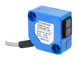
AutomationDirect photoelectric sensor, rectangular, diffuse, infrared, 600mm sensing distance, light-on, PNP, potentiometer, 1 kHz switching frequency, plastic housing, pigtail.
