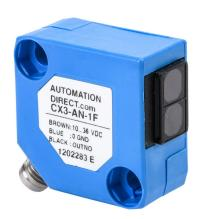
AutomationDirect photoelectric sensor, rectangular, diffuse, infrared, 600mm sensing distance, light-on, NPN, potentiometer, 1 kHz switching frequency, plastic housing, 3-pin M8 quick-disconnect.
