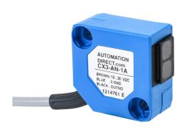
AutomationDirect photoelectric sensor, rectangular, diffuse, infrared, 600mm sensing distance, light-on, NPN, potentiometer, 1 kHz switching frequency, plastic housing, pigtail.
