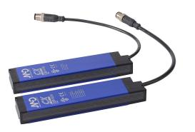
Micro Detectors CX light grid, sender/receiver pair, measuring, 10mm resolution, 160mm detection height, 0.3-6m operating distance, PNP, 0-10 VDC analog output, configurable, (1) 4-pin and (1) 8-pin M12 quick-disconnect.
