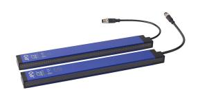
Micro Detectors CX light grid, sender/receiver pair, measuring, 5mm resolution, 320mm detection height, 0.1-3m operating distance, PNP, 0-10 VDC analog output, configurable, (1) 4-pin and (1) 8-pin M12 quick-disconnect.
