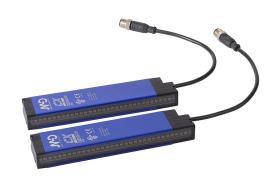
Micro Detectors CX light grid, sender/receiver pair, measuring, 5mm resolution, 160mm detection height, 0.1-3m operating distance, PNP, 0-10 VDC analog output, configurable, (1) 4-pin and (1) 8-pin M12 quick-disconnect.
