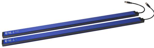
Micro Detectors CX light grid, sender/receiver pair, measuring, 10mm resolution, 800mm detection height, 0.3-6m operating distance, PNP, 4-20 mA analog output, configurable, (1) 4-pin and (1) 8-pin M12 quick-disconnect.
