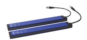
Micro Detectors CX light grid, sender/receiver pair, measuring, 10mm resolution, 320mm detection height, 0.3-6m operating distance, PNP, 4-20 mA analog output, configurable, (1) 4-pin and (1) 8-pin M12 quick-disconnect.
