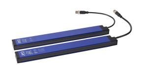
Micro Detectors CX light grid, sender/receiver pair, measuring, 10mm resolution, 320mm detection height, 0.3-6m operating distance, PNP, 4-20 mA analog output, configurable, (1) 4-pin and (1) 8-pin M12 quick-disconnect.
