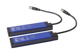
Micro Detectors CX light grid, sender/receiver pair, measuring, 5mm resolution, 160mm detection height, 0.1-3m operating distance, PNP, 4-20 mA analog output, configurable, (1) 4-pin and (1) 8-pin M12 quick-disconnect.
