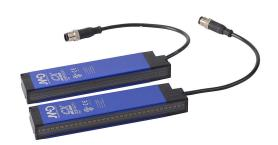
Micro Detectors CX light grid, sender/receiver pair, object detection, 5mm resolution, 160mm detection height, 0.3-3m operating distance, PNP, (1) 4-pin and (1) 5-pin M12 quick-disconnect.
