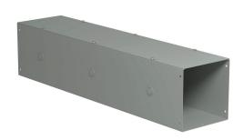
Hammond CW series lay-in wireway, 8 x 8 x 36in, carbon steel, ANSI 61 gray, powder coat finish, with knockouts, NEMA 1.
