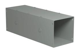
Hammond CW series lay-in wireway, 8 x 8 x 24in, carbon steel, ANSI 61 gray, powder coat finish, with knockouts, NEMA 1.
