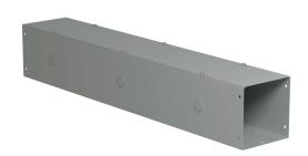
Hammond CW series lay-in wireway, 6 x 6 x 36in, carbon steel, ANSI 61 gray, powder coat finish, with knockouts, NEMA 1.
