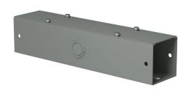
Hammond CW series lay-in wireway, 2.5 x 2.5 x 12in, carbon steel, ANSI 61 gray, powder coat finish, with knockouts, NEMA 1.
