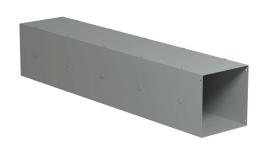
Hammond CW series lay-in wireway, 12 x 12 x 60in, carbon steel, ANSI 61 gray, powder coat finish, with knockouts, NEMA 1.
