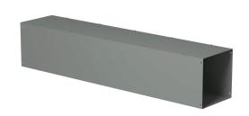
Hammond CW series lay-in wireway,  $12 \times 12 \times 60$  in, carbon steel, ANSI 61 gray, powder coat finish, NEMA 1.
