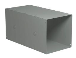
Hammond CW series lay-in wireway, 12 x 12 x 24in, carbon steel, ANSI 61 gray, powder coat finish, with knockouts, NEMA 1.
