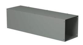
Hammond CW series lay-in wireway,  $10 \times 10 \times 36$ in, carbon steel, ANSI 61 gray, powder coat finish, NEMA 1.
