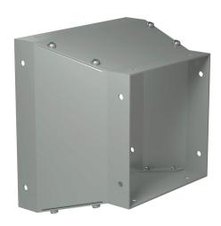
Hammond CW series lay-in wireway fitting, reducer,  $8 \times 8$  in to  $6 \times 6$  in, carbon steel, ANSI 61 gray, powder coat finish, NEMA 1. For use with CW series wireway.
