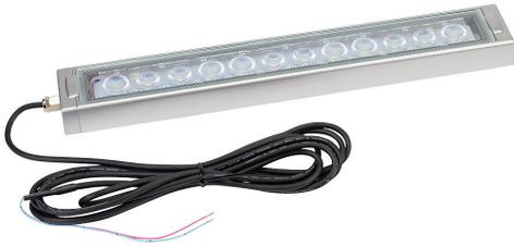
Patlite LED light bar, 300mm length, 24 VDC operating voltage, daylight white, bracket mount, pigtail, aluminum body, 9.8ft/3m cable length, IP66 and IP67. Mounting bracket included.
