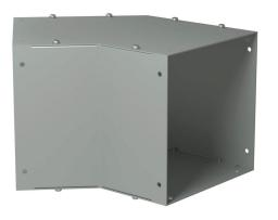
Hammond CW series lay-in wireway fitting, 45-degree elbow, 8 x 8in, carbon steel, ANSI 61 gray, powder coat finish, NEMA 1. For use with CW series wireway.
