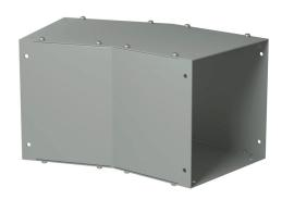
Hammond CW series lay-in wireway fitting, 22.5-degree elbow, 8 x 8in, carbon steel, ANSI 61 gray, powder coat finish, NEMA 1. For use with CW series wireway.
