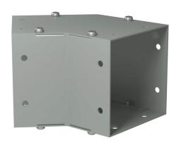
Hammond CW series lay-in wireway fitting, 45-degree elbow, 4  $\times$  4in, carbon steel, ANSI 61 gray, powder coat finish, NEMA 1. For use with CW series wireway.
