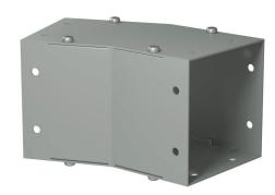
Hammond CW series lay-in wireway fitting, 22.5-degree elbow, 4 x 4in, carbon steel, ANSI 61 gray, powder coat finish, NEMA 1. For use with CW series wireway.
