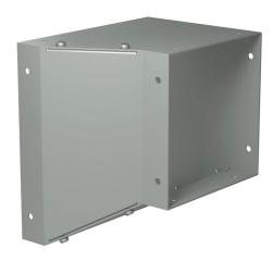
Hammond CW series lay-in wireway fitting, corner reducer, 8 x 8in to 6 x 6in, carbon steel, ANSI 61 gray, powder coat finish, NEMA 1. For use with CW series wireway.
