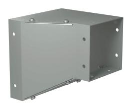
Hammond CW series lay-in wireway fitting, corner reducer, 6 x 6in to 4 x 4in, carbon steel, ANSI 61 gray, powder coat finish, NEMA 1. For use with CW series wireway.
