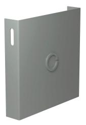
Hammond CW series lay-in wireway fitting, cover plate, 6 x 6in, carbon steel, ANSI 61 gray, powder coat finish, with knockouts, NEMA 1. For use with CW series wireway.
