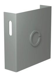
Hammond CW series lay-in wireway fitting, cover plate,  $4 \times 4$ in, carbon steel, ANSI 61 gray, powder coat finish, with knockouts, NEMA 1. For use with CW series wireway.
