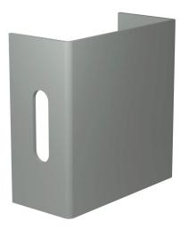
Hammond CW series lay-in wireway fitting, cover plate,  $2.5 \times 2.5$  in, carbon steel, ANSI 61 gray, powder coat finish, NEMA 1. For use with CW series wireway.
