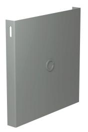
Hammond CW series lay-in wireway fitting, cover plate, 10 x 10in, carbon steel, ANSI 61 gray, powder coat finish, with knockouts, NEMA 1. For use with CW series wireway.
