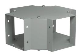
Hammond CW series lay-in wireway fitting, cross fitting, 4 x 4in, carbon steel, ANSI 61 gray, powder coat finish, NEMA 1. For use with CW series wireway.
