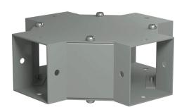
Hammond CW series lay-in wireway fitting, cross fitting, 2.5 x 2.5in, carbon steel, ANSI 61 gray, powder coat finish, NEMA 1. For use with CW series wireway.
