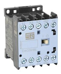
WEG Electric CWC series IEC miniature contactor, 9A, (3) N.O. power poles, (1) N.O. auxiliary contacts, 480 VAC (60Hz) coil voltage.
