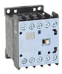
WEG Electric CWC series IEC miniature contactor, 9A, (3) N.O. power poles, (1) N.O. auxiliary contacts, 24 VAC (60Hz) coil voltage.
