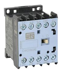
WEG Electric CWC series IEC miniature contactor, 9A, (3) N.O. power poles, (1) N.C. auxiliary contacts, 120 VAC (60Hz)/110 VAC (50Hz) coil voltage.
