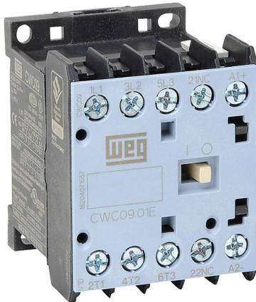
WEG Electric CWC series IEC miniature contactor, 9A, (3) N.O. power poles, (1) N.C. auxiliary contacts, 24 VAC (60Hz) coil voltage.
