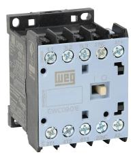
WEG Electric CWC series IEC miniature contactor, 9A, (3) N.O. power poles, (1) N.C. auxiliary contacts, 24 VDC coil voltage, low consumption.
