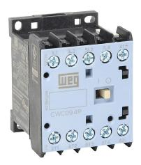
WEG Electric CWC series IEC miniature contactor, 9A, (4) N.O. power poles, 480 VAC (60Hz) coil voltage.
