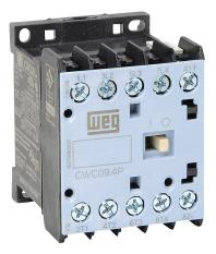
WEG Electric CWC series IEC miniature contactor, 9A, (4) N.O. power poles, 24 VAC (60Hz) coil voltage.
