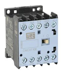
WEG Electric CWC series IEC miniature contactor, 7A, (3) N.O. power poles, (1) N.O. auxiliary contacts, 480 VAC (60Hz) coil voltage.
