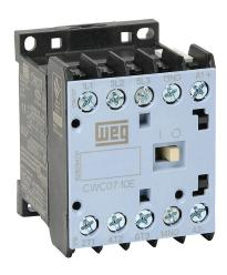
WEG Electric CWC series IEC miniature contactor, 7A, (3) N.O. power poles, (1) N.O. auxiliary contacts, 208-240 VAC (60Hz) coil voltage.
