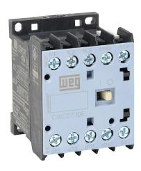
WEG Electric CWC series IEC miniature contactor, 7A, (3) N.O. power poles, (1) N.O. auxiliary contacts, 120 VAC (60Hz)/110 VAC (50Hz) coil voltage.
