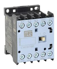
WEG Electric CWC series IEC miniature contactor, 7A, (3) N.O. power poles, (1) N.O. auxiliary contacts, 24 VAC (60Hz) coil voltage.
