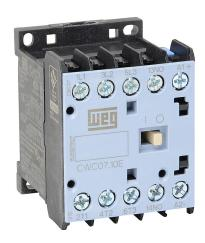
WEG Electric CWC series IEC miniature contactor, 7A, (3) N.O. power poles, (1) N.O. auxiliary contacts, 24 VDC coil voltage, low consumption.
