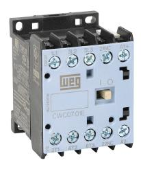
WEG Electric CWC series IEC miniature contactor, 7A, (3) N.O. power poles, (1) N.C. auxiliary contacts, 480 VAC (60Hz) coil voltage.
